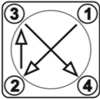
Figure 3 - Screw tightening sequence
