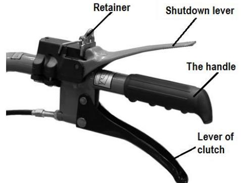
**Motor Shutdown Switch****TILLER MAINTENANCE**
