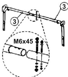
3. Install the side leg bows (part 8) on both sides between the front and rear supports, securing them with M6x45 bolts and M6 nuts.
