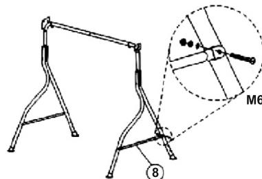
5. Attach the rear leg assembly to the rear supports using M6x60 bolts and M6 nuts.
