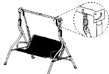
2. Attach the rear support (part 2) and the front support (part 1) to the upper support assembled earlier using M8x85 bolts - M8 nuts and M6x80 bolts - M6 nuts respectively. Install the foot-rests (part 21) on the supports.
