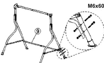
7. Attach the side rails at the base of the seat with M6x55 bolts and M6 nuts.
